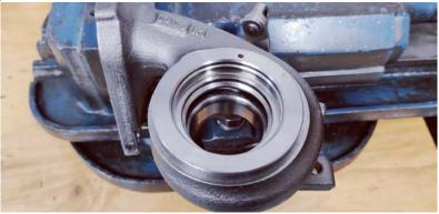
8. The Super Cores can now be installed, NOTE the alignment pins and the correct housing for each side as follows. (Rear turbo has a tab with tapped hole on the turbine housing inlet flange)
