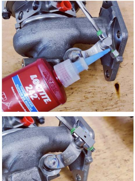
13. When wastegate adjustments are set correctly, torque the lower adjustment nut to 85 Inch-lbs use blue Loctite. Then install the locking circlips.
