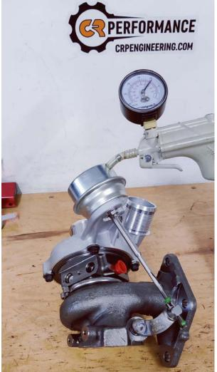
12. The wastegate puck should just start to free from the housing at this 9-9.5 inHg. Check by cycling from 15 inHg down to 0 slowly, motion of the lever should stop at 9-9.5 inHg.
