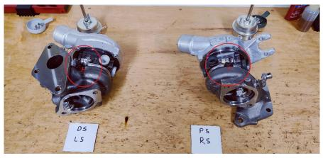
5. Remove the V Band Clamps on each turbo and use a suitable penetrating oil if the housings are not free for ~15-30 Minutes.
