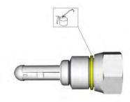
13. Install and tighten the new turbocharger fitting, oil filter assembly into the engine block.
