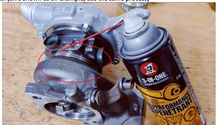
6. Using a dead blow or rubber mallet remove the cartridges from the turbine housings. Tap evenly during removal on all sides. Heat may be needed on older units, if so, heat the turbine housing with a propane torch at low heat for 2-5 Min at the joint to aid in removal.
