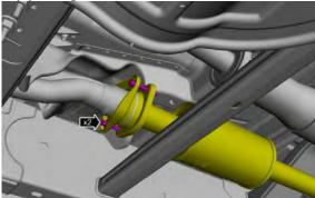
5. Remove the LH catalytic converter nuts and discard.
