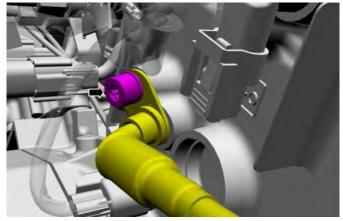
12. Remove the turbocharger mounting bolts, then remove the turbocharger.
