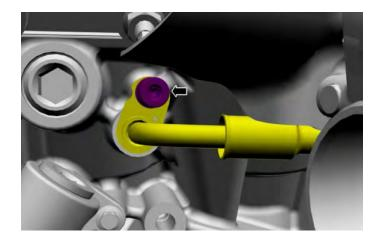
11. Install and evenly tighten the new left turbocharger exhaust flange nuts.
