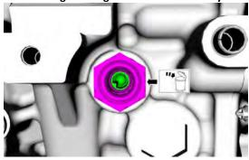
7. Remove the turbocharger oil return tube bolts, then remove and discard the turbocharger oil return tube.
