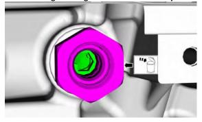
3. Remove the turbocharger oil return tube bolts, then remove and discard the turbocharger oil return tube.
