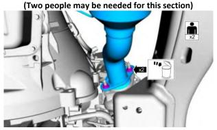
NOTE: The below following steps are only required if servicing the exhaust manifold adaptors, this can be done later with the turbochargers removed if wished or can be done at this time with the turbochargers mounted.
