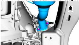
5. Position the LH catalytic converter in vehicle. Install the LH catalytic converter nuts.
