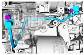
6. Remove and discard the turbocharger fitting and oil filter assembly from the engine block.
