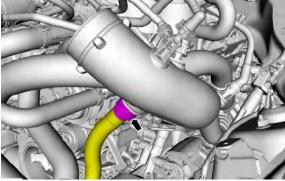
4. Install the air cleaner outlet pipe RH. Torque: 44 lb.in (5 Nm)
