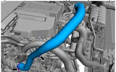
5. Disconnect the bypass valve tube LH.
