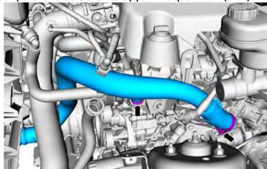
9. Loosen the clamps and remove the CAC intake pipe RH. Torque: 44 lb.in (5 Nm)
