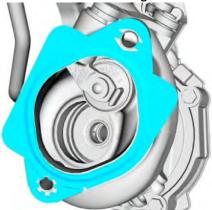
2. If removed, install and tighten the turbocharger exhaust flange and the turbocharger exhaust flange stud / bolts. Torque: 30 lb.ft (40 Nm)
