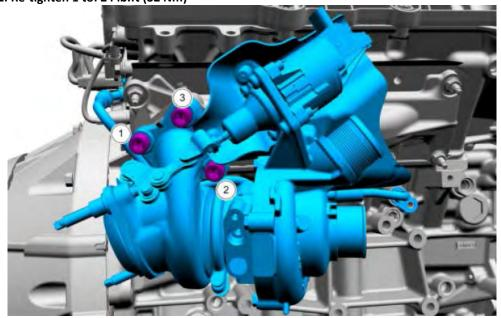
8. Install and tighten the turbocharger coolant return tube bolt.
