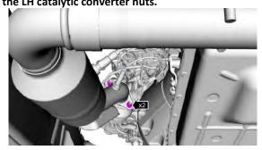
6. Tighten the clamp. Torque: 41 lb.ft (55 Nm)
