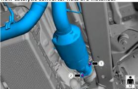
9. Install the muffler inlet pipe flange bolts. (Torque: 30 lb.ft (40 Nm))
