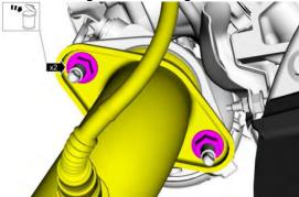
6. Remove the turbocharger coolant supply tube bolt, then disconnect the turbocharger coolant supply tube.
