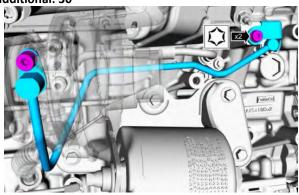
16. Install the air conditioning compressor, and then tighten the air conditioning compressor mounting bolts.
