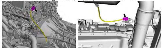
3. Disconnect the RH HO2S pushpins and electrical connectors.
