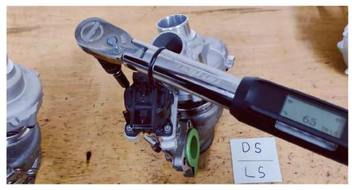
12. The super cores are now installed finalizing the complete upgraded turbochargers. Install removed heat shields and torque heat shield hardware to 65 Inch-Lbs. These are then ready to install with standard installation instructions in the next section.
