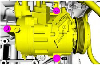
17. Connect the air conditioning compressor electrical connectors and the harness retainer.
