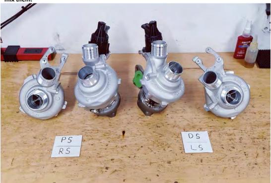
2. Remove the wastegate circlips from both sides on the turbine end.
