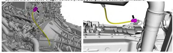
11. Connect the RH HO2S pushpins and electrical connectors.
