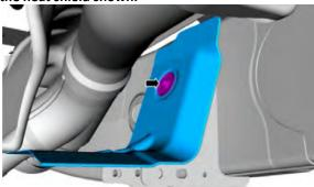
7. Loosen the clamp and remove the LH catalytic converter.
