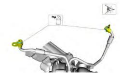
12. Remove and discard the turbocharger gasket.
