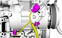
4. Loosen the air conditioning compressor mounting bolts and position the air conditioning compressor aside.
