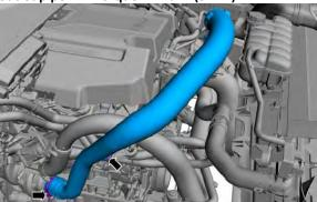
5. Install the retainers and position the wiring harness.
