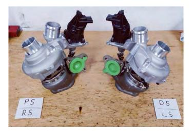
13. We recommend pre-oiling of the turbo inlets as shown before final installation, add a small amount of oil before oil line installation. (2.7L Shown as an example, use the same process)
