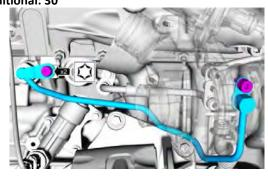
17. Lubricate the new turbocharger oil return tube O-ring seals with clean engine oil
