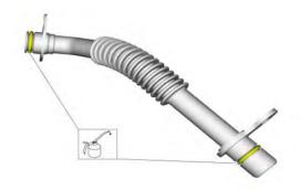
21. Fully seat the turbocharger oil return tube into the turbocharger and engine bore holes flush to 2.5 mm off of the mounting surface prior to fastener rundown. Install new the turbocharger oil return tube, then install and tighten the turbocharger oil return tube bolts.
