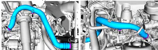
2. Install the air cleaner outlet pipe LH. Torque: 44 lb.in (5 Nm)
