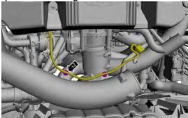
6. Install the air cleaner outlet pipe. Torque: 44 lb.in (5 Nm)
