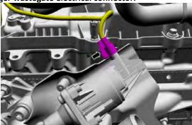
12. Lubricate the new turbocharger fitting and oil filter assembly O-ring seal with clean engine oil.
