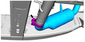
8. Remove the RH catalytic converter nuts and discard. Remove the RH catalytic converter.
