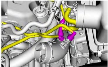
7. Loosen the clamp and remove the air cleaner outlet pipe LH. Torque: 44 lb.in (5 Nm)
