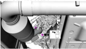
6. Remove RH bolt and the heat shield shown.
