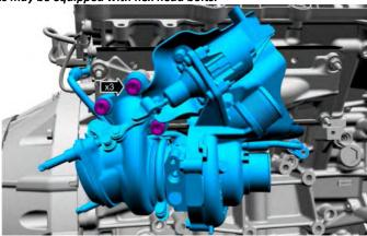
13. Remove and discard the turbocharger coolant supply and the turbocharger coolant return tube O-ring seals.
