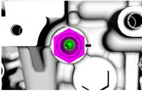
14. Lubricate the new turbocharger oil supply tube O-ring seal with clean engine oil.
