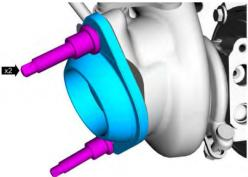
3. Install the new turbocharger gasket by pressing the gasket into the turbocharger flange groove evenly until at least 50% of the gasket is within the groove.
