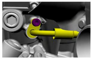
7. Release the fuel tubes from the retainers, then position the fuel tubes out of the way.
