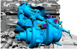
10. Remove and discard the turbocharger coolant supply and the turbocharger coolant return tube O-ring seals.
