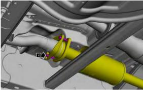
10. Connect the LH Heated Oxygen Sensors (HO2S) pushpin and electrical connectors.
