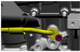
11. Remove the turbocharger coolant return tube bolt, then disconnect the turbocharger coolant return tube.
