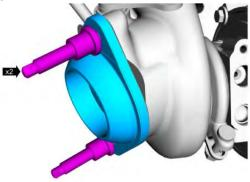
3. Install the new turbocharger gasket by pressing the gasket into the turbocharger flange groove evenly until at least 50% of the gasket is within the groove.
