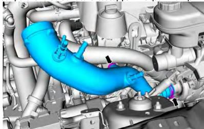
8. Loosen the clamp and remove the CAC intake pipe LH. Torque: 44 lb.in (5 Nm)
