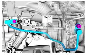
2. Remove and discard the turbocharger fitting and oil filter assembly from the engine block.
