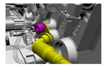
9. Install and tighten the turbocharger coolant supply tube bolt.
