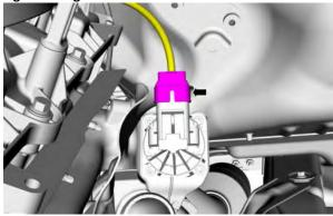
Lubricate the new turbocharger fitting and oil filter assembly O-ring seal with clean engine 13. oil.
