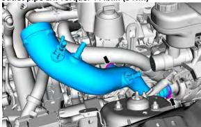
3. Connect the quick release couplings & the bypass valve tube LH.
