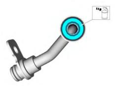
6. Install the new turbocharger coolant supply and the new turbocharger coolant return tube O-ring seals Lubricate the new O-ring seal with clean engine coolant.
