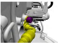
9. Remove the turbocharger mounting bolts, then remove the turbocharger.
