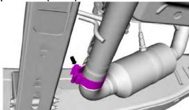
7. Install the LH catalytic converter nuts. Tighten Nuts in 1-2-1 sequence.
