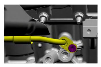
10. Install and evenly tighten the new left turbocharger exhaust flange nuts.
