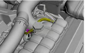
2. Loosen the clamps and remove the air cleaner outlet pipe. Torque: 44 lb.in (5 Nm)
