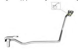
15. Install the new turbocharger oil supply tube, verify the correct assembly by pulling back on the turbocharger fitting, oil filter assembly tube end. Then install and tighten the turbocharger oil supply tube bolts.
