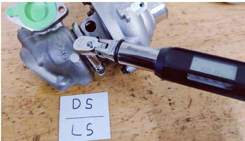
**IMPORTANT NOTICE:** Failure to seat the CHRA correctly and torque the V Band nuts to specification can cause damage or failure of the turbocharger, this type of damage is not covered by warranty.
