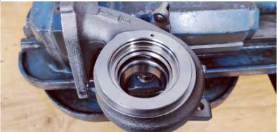
8. The Super Cores can now be installed onto the stock housings, NOTE the alignment pins and the correct housing for each side as follows. Install carefully not to damage the turbine wheels blades.
