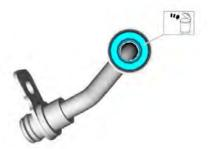
6. Install the new turbocharger coolant supply and the new turbocharger coolant return tube O-ring seals Lubricate the new O-ring seal with clean engine coolant.
