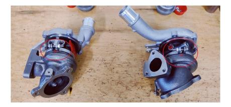
5. Remove the V Band Clamps on each turbo and use a suitable penetrating oil if the housings are not free for ~15-30 Minutes.
