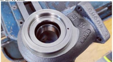
8. The Super Cores can now be installed, NOTE the alignment pins and the correct housing for each side as follows. (Rear turbo has a tab with tapped hole on the turbine housing inlet flange)
