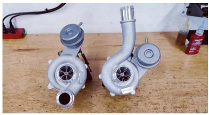
15. We recommend pre-oiling of the turbo inlets as shown before final installation, add a small amount of oil before oil line installation.
