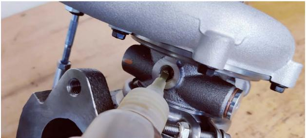
**IMPORTANT NOTICE:** Failure to seat the CHRA correctly and torque the V Band nuts to specification can cause damage or failure of the turbocharger, this type of damage is not covered by warranty.
