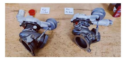
11. Set the wastegates to open at 2.5-3.5 PSI applied to the actuator, this can be done with a quality regulator on a compressor, or any other means to accurately apply pressure to the actuators. The wastegate puck should just start to free from the housing at this 2.5-3.5 PSI.
