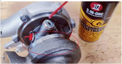
6. Using a dead blow or rubber mallet remove the cartridges from the turbine housings. Tap evenly during removal on all sides. Heat may be needed on older units, if so, heat the turbine housing with a propane torch at low heat for 2-5 Min at the joint to aid in removal.
