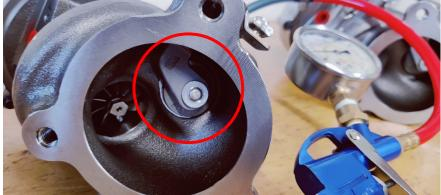
13. When pressures are set correctly, torque the lower adjustment nut to 65 Inch-lbs use blue Loctite. Then install the locking clips.
