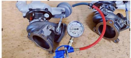
12. The wastegate puck should just be starting to lift at 2.5-3.5 PSI you can tap it with a finger to confirm when it frees as you adjust the wastegate pressure. Duplicate these past two steps for the other turbo.
