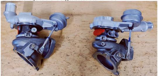
2. Remove the wastegate circlips.
