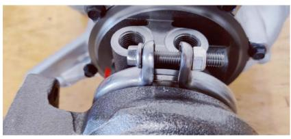
**IMPORTANT NOTICE:** Failure to seat the CHRA correctly and torque the V Band nuts to specification can cause damage or failure of the turbocharger, this type of damage is not covered by warranty.
