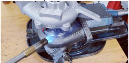
7. Once cartridges have been removed, clean the turbine housing interface with brake cleaner or suitable solvent until a clean metal surface is seen, if needed a minimal amount of sanding with a 200 or higher grit sand paper can be used.
