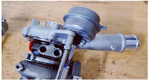
4. Mark the V Band Clamp bolt positions on the turbine housings using an engraver or marker for alignment in reassembly.
