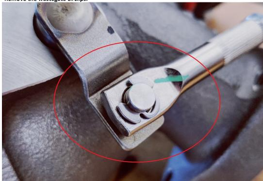
3. Remove the wastegate mounting nuts and remove the wastegates. (Note Rear & Front actuators are different do not mix banks)
